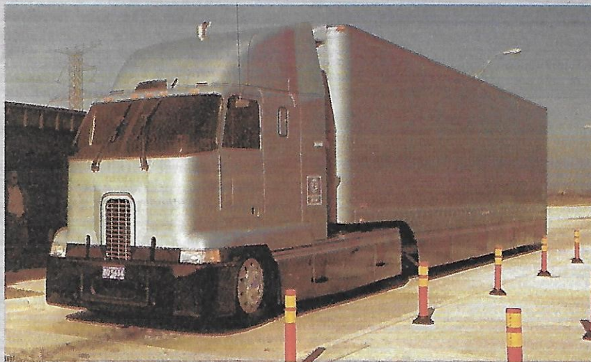
Futuristic DDA tractor-trailer, powered by 300-hp. DDEC (electronically controlled) engine, produced 7.84 mpg in 392-mi. test through Michigan and Indiana.
