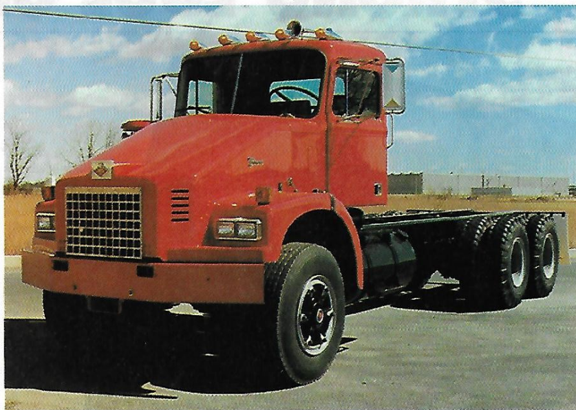
Deutz-powered Diamond Reos have wedge-shaped hoods, cutting aerodynamic drag. The sharp hood angle is possible because the engine is air-cooled and has no radiator.
