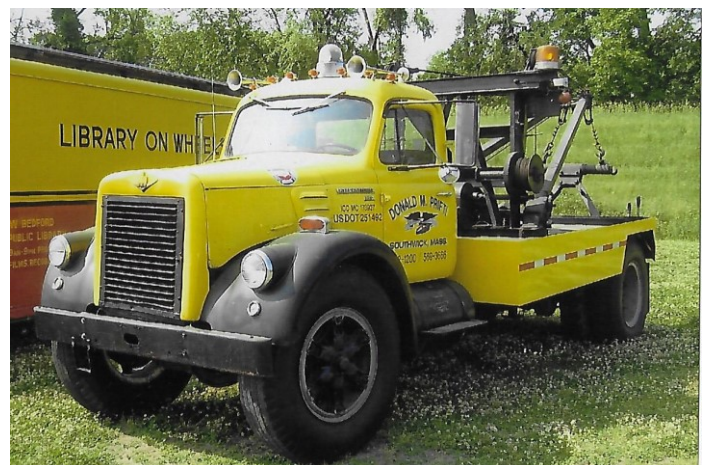
1961 International V-210 549 cubic inch engine with a Holmes W-35 with a Shop-Built Body
