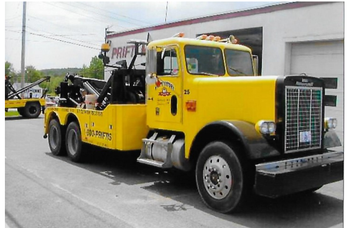
1977 White-Freightliner WFC 12064 Cummins VT-903 with a Holmes Super-Star Body with a 1625 Lift
