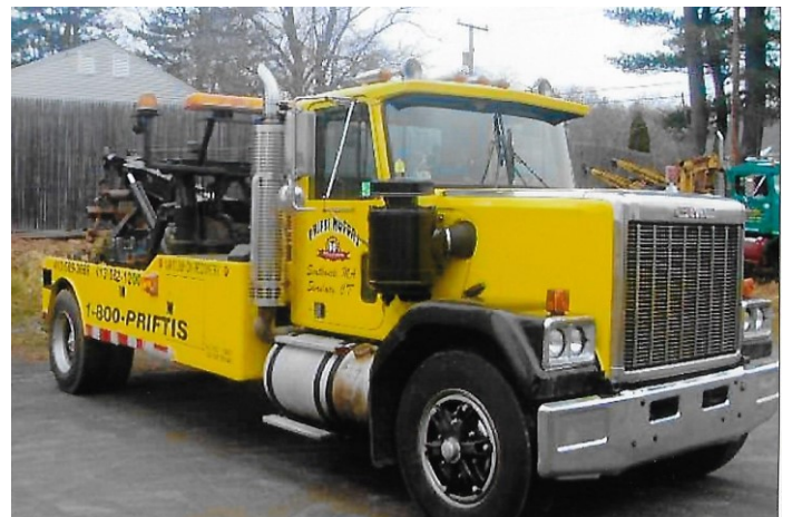
1978 GMC General with a Detroit Diesel 6V-92. The Body is a 1625 with a Zack Lift.
